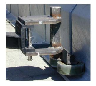
When the incident is in a construction zone a fourth option is to use a piece of construction equipment such as a backhoe or front end loader in conjunction with a set of barrier lifting tongs to reposition the wall to its original location. Because each module only weighs 1500 pounds (approximate) many different kinds of construction equipment can be used when required to "push" the wall back into approximate position and minimize work zone disruption.
